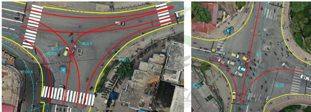
Figure 3: Sample of Negotiation Distance and Radius Measurement
